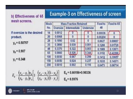
Here this would be the product, this would be the feed and this would be the reject. So  $y_A$ ,  $_{yB}$  and  $y_C I$  can calculate over here and similarly I can calculate the effectiveness of screen. So for 65 I am getting 59.76% as.
