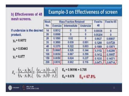
Similarly we can calculate effectiveness of 48 mesh screen if undersize is a desired product so undersize to 48 this is the region where we have to focus, so this is  $y_{C}$ , this is  $y_{B}$ , and this is  $y_{A}$ , summation of these three will give the value and using these value in this expression we can have the effectiveness of screen which comes out as 67.8%. And here we have to calculate the effectiveness of 65 mesh screen if oversize the desired product following similar method.
