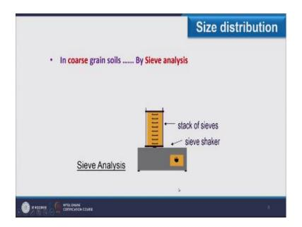
In coarse grain soils by sieve analysis, what is the meaning of this, that coarse grain size distribution we carry out using sieve analysis. However if you see the data or see mesh chart it gives the value up to 40, up to 40  $\mu$ m only so sieve analysis does not give the size distribution below 40  $\mu$ m so when we have to compute the distribution below this.
