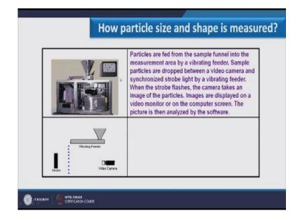
By a vibrating feeder, when the strobe flashes the camera takes the image of the particle and this image are displayed on the associated computer and the picture is then analyzed by the software. So if you see this particular image which is reflected on a computer screen this is basically the pictures taken by this video camera. So after a short interval continuously these images are coming and we can analyze this.
