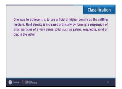
It that is to change the density or to carry out separation is to use a fluid of higher density as the settling media. Fluid density is increased artificially by forming as a suspension of a small particles of very dense solid such as galena, magnetite, sand or clay in the water so we can change the density of the fluid of the media and so that the settling ratio can be changed.
