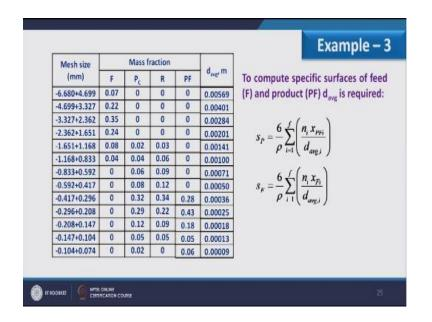
Next value of n we have to calculate, once I know  $d_{avg}$  the value of n should be calculated next to it, how I can calculate value of  $n_i$ , the  $n_i$  is basically specific surface ratio for i<sup>th</sup> intervals so for each interval I can calculate this, how I can calculate this using the value of.
