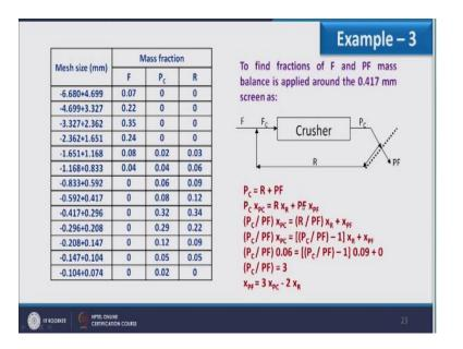
So to find fraction of F as well as PF mass balance is applied around 0.417 mm screen. Because F is given to us and fraction of F are already known to us we have to calculate fraction of PF. So we will make the balance over here where  $P_C$  is equal to PF=R. So  $P_C$ =R+PF, when we make the component balance  $P_C \ge R X_R + PF X_{PF}$ , we have to calculate  $X_{PF}$  for different fractions.
