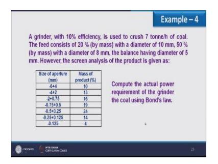
7 ton per hour of coal, the feed consists of 20% by mass with diameter of 10mm, 50% by mass with diameter of 8mm, and balance having the diameter of 5mm. However the screen analysis of the product is given in this table, what we have to compute is actual power consumption of the grinder using Bond's law, so here you see the efficiency of grinding is given to us we have to calculate actual power consumption, so as far as.
