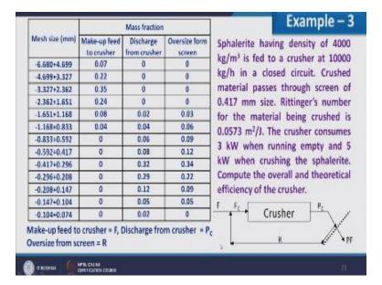
Now if you consider this diagram 10,000 is a feed to closed circuit. So when we consider the closed circuit obviously F would be the feed which we have considered as 10,000 kg/h. Crushed
