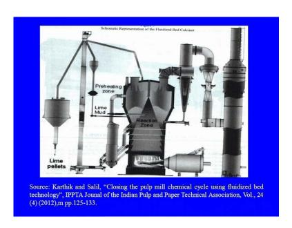
This is the fluidised bed actually the lime kiln that you are having for the preheating the lime mud that is going to the fluidized bed and so this some of the problems, which are inherent in case of the lime kiln that is eliminated here with and finally, we are getting the lime. So, that lime again that can be used and this is the new development that is taking place in case of the lime sludge reburning, otherwise the earlier it was the rotary kiln that was been used.
