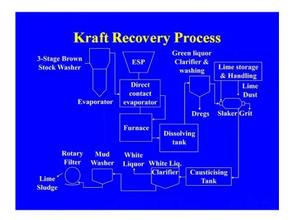
So, in order to have now we are having the 4 stage brown stock washer and from there after the brown stack washer the black liquor actually here the black should be black liquor from the your 3 stage or the 4 stage brown washer that is going through evaporators that as I told you that is normally we having the long tube evaporator in case of the karft recovery process with the backward feed arrangement because you are not the forward feed because it will become highly viscous.
