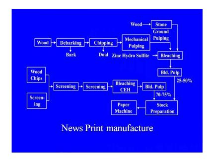
This, is the news print manufacture where we are using wood that is going to the both the mechanical and the chemical it may be sequence now it is the not the CE, but CEHH or it may be the DEH, which the chlorine dioxide or it may be oxygen delignification also.
