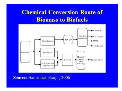
This is the chemical conversion route for the biomass gasification that is the biomass gasification pyrolysis or hydrothermal liquefaction; that may be there in presence of hydrogen. We may get the synthesis gas that the from the synthesis gas you can go for the FT diesel DME dimethyl ether or the methane and the bio oil hydro treating and refining then the hydrocarbon. So, this is the process that can be used for the gasification of the biomass.
