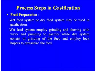
Now, let us discuss what are the in detail about the various steps in gasification feed preparation, wet feed system or dry feed system may be used in the gasification. Wet feed system employ grinding and slurring with the water and pumping to the gasifier while dry system consist of grinding of the feed and empty lock hopers to pressurize the feed and so always the dry actually the a raw material that will be the more economical than the by your the wet feed.
