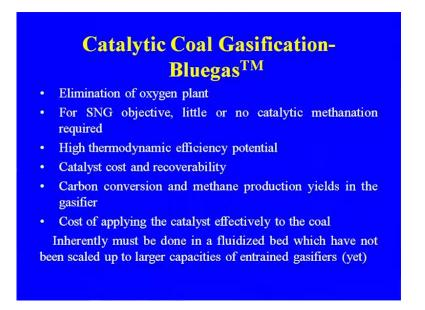
So, elimination of the oxygen for SNG of objective syngas little or no catalytic methanation required high thermodynamic efficiency catalyst cost and recoverability, carbon conversion and methane production yields in the gasifier. So, cost of the applying the catalyst effectively with coal inherently must be done in fluidized bed which have not been scaled up to the larger capacity.
