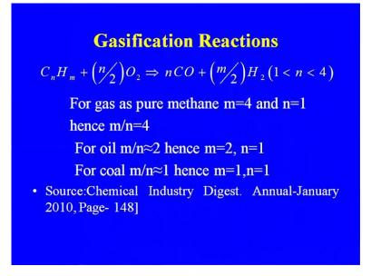
These are the some of the series of the reaction because you see the partial oxidation or the steam reforming that is a complex initial.
