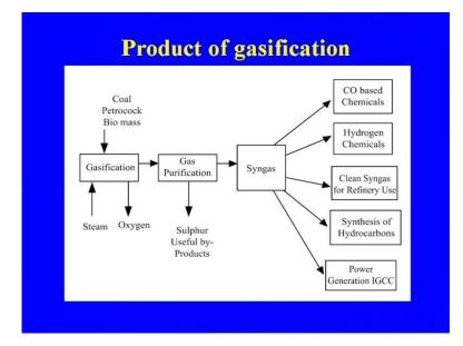
Process steps in the gasification. Some of the process steps involved in case of the gasification first part is the feed preparation. Then the gasification, gasification in the presence of air and the presence of oxygen because many of the plant they are having the
