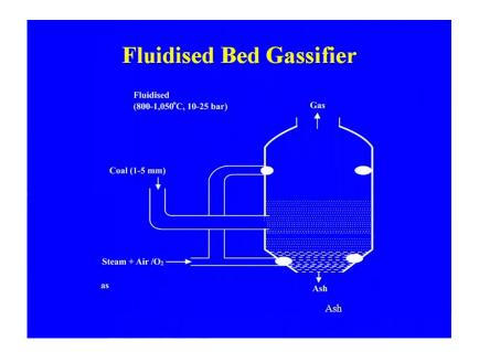
This is the again another type of the fluidized bed gasifier where the fluidization is taking place and syngas after going to the cyclone where the particulate matters are separated and then the syngas that will go for further processing.
