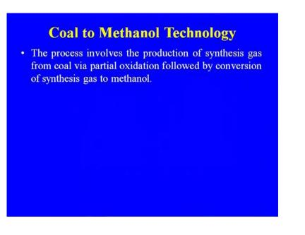
Coal to methanol technology, the process involves the production of synthesis gas from coal via partial oxidation followed by conversion of the synthesis gas to methanol, this is the technology that is been used for the production of the methanol. Again we will be discussing in detail about the production of the methanol from the synthesis gas, while discussing about the petro chemicals in module 6, module 7 sorry.
