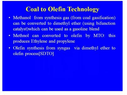
Coal to olefin technology, methanol from synthesis gas from coal gasification can be converted to dimethyl ether using bifunction catalyst, which can be used as a gasoline blend or methanol can be converted to olefin by MTO process. This this process produces ethylene and the propylene, olefin synthesis from synthesis gas via dimethyl ether to olefin process, that is also SDTO that is that is also available.
