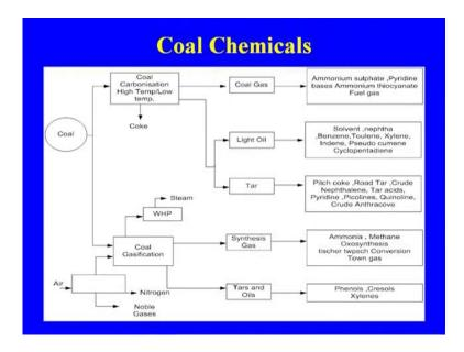
Coal, coal carbonization, high temperature, low temperature carbonization because two types of the carbonization were taking and we are getting the coke and the gases, and the coal tar that we are using for the production of the your various actually, the inorganic and organic compound. Ammonium sulphate that is one of the very important part of the any steel making plant, because in many of the steel plant, they are making the ammonium sulphate or ammonium nitrate.
