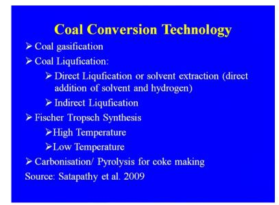
Coal conversion technology coal gasification, coal liquification, that may be direct liquification or the solvent extraction where the, we are adding the solvent and hydrogen, indirect liquification. Fischer Tropsch synthesis, that may be again high temperature and low temperature, carbonisation pyrolysis of the for coke making. As I told you earlier also, that the calcium carbide and acetylene that was the major source of making many of the chemicals or now, we called the petro chemical.
