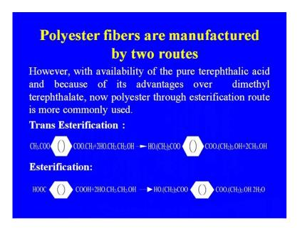
So, as I told you that we are having the two routes. One is this DMT route another is your terephthalic acid purified terephthalic acid route. So, the transesterification or the esterification reaction that is taking place. In one case that we are getting the methanol as a byproduct but, another case only the water is coming. So, this is the difference between
