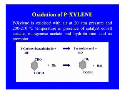
This is the reaction that is taking place in case of the Paraxylene. That is in the presence of air that is oxidized at this Para xylene is oxidized with air at twenty atmosphere pressure in presence of the catalyst cobalt acetate, manganese acetate and hydrobronic acid as a promoter.
