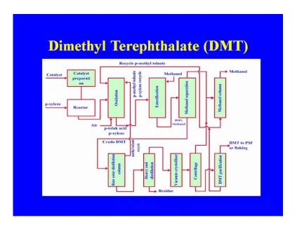
This is the process before going to the process for dimethyl terephthalate that is the Para xylene that is going to the catalyst preparation section. Then Para xylene that is going to the reaction section oxidation esterification where methanol and here as i told you during the process methanol again, it is been generated in the reaction and the final that the DMT that is going for the polyester plant for making of the polyester that is the polymerization of the d m t.
