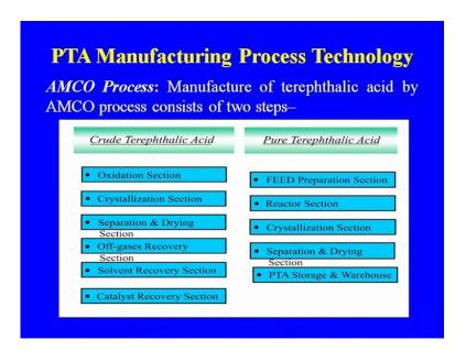
This is the AMCO process oxidation crystallization separation and drying, off gases recovery, solvent recovery, catalyst recovery and this is for purifying the feed
