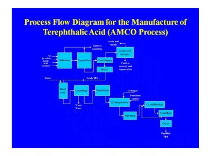
These are the two another process that has been developed. That is the Henkel process or the Henkel two processes, this is the AMCO process in more detail that as I told you we are having the oxidation crystallizer centrifuging. Then again wash tank centrifuging hydrogenation for removal of the impurities filtration. Again crystallization centrifuging and drying so, this part is for the removal of the impurities which is present there
