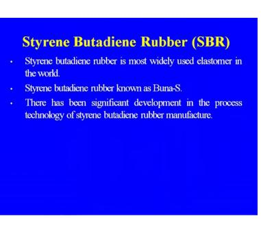
So, styrene butadiene rubber is known as BUNA-S, also there has been significant development in the process technology of the styrene butadiene rubber manufacture. Amongst the various processes which we are using emulsion polymerization of the styrene butadiene rubber is most commonly used method.
