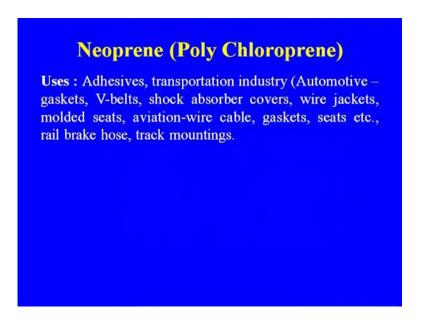
So, these are the some of the major application of the polychloroprene again here also the same acetylene route is available. So, that can be made from the acetylene or the butadiene route because earlier when the butadiene was not from the petrochemical. So, acetylene that was a route for making of the chloroprene, So acetylene route involves dimerization of the acetylene to monovinyl acetylene followed by the reaction of monovinyl acetylene with H C L.
