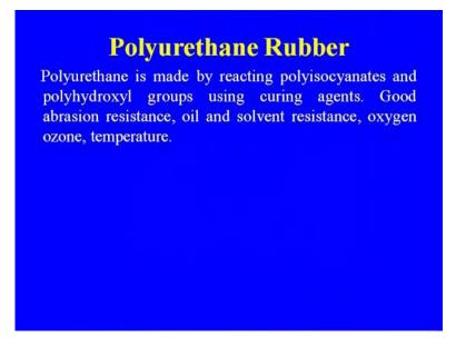
Polyisocyanates and polyhydroxyl group using curing agents, good abrasion resistance oil and solvent resistance oxygen ozone resistance and the temperature resistance. So, this is the actually the some of the characteristics of the polyurethane rubber. (Refer Slide Time: 37:11)
