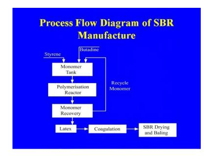
This is the process for the manufacture of S B R. The styrene butadiene that is going to the monomer tank mixing and the polymerization reactor where the reaction that is taking place and as I told you the after the completion 60 75 percent of the completion, that is going to the monomer recovery where the monomer again. It is recovered here. That is going to recycling and we are getting the latex as such it can be used or it will go for the coagulation.
