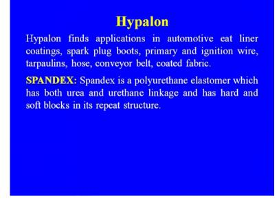
We called for the lining that sometimes. We are using earlier, it was very common use of the tarpaulins was there hose, conveyor, belt coated fabrics. Another class of the synthetic rubber that is spandex is a polyurethane elastomer which has both urea and urethane linkage and has hard and soft blocks in its repeat structure.
