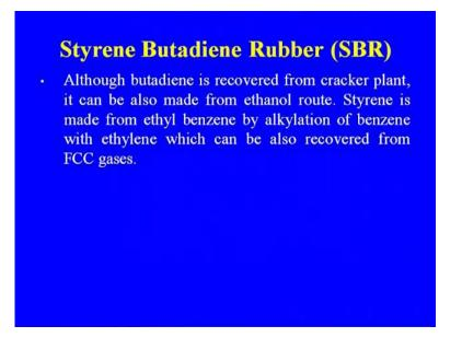
Although butadiene again is recovered from the cracker plant it can be also made from the ethanol route styrene is made from the ethyl benzene by alkylation of benzene with ethylene which can be also recovered from the F C C gases. I told you that the now the interest is there why not to recover that ethylene which is available in the F C C gases .
