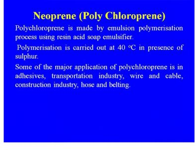
Polymerization is carried out at forty degree centigrade in presence of the sulfur. Some of the major application of the poly chloroprene is in adhesive transportation industry wire and cable construction, industry hose and belting uses adhesive transportation, automotive gaskets, v-belts, shock absorber covers wire, jackets, molded seats, aviationwire cable, gaskets, seats etcetera rail brake hose track mounting.
