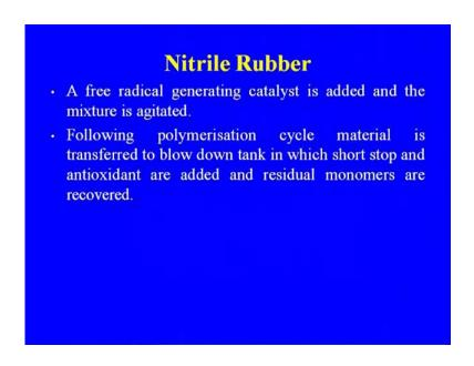
The mixture is agitated following polymerization cycle material is transferred to the blow down tank in which the short stop and the antioxidants which are added and residual monomer are recovered and this is again a recycle to the reactor.
