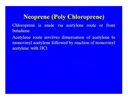
So, this was the method that was developed earlier with the for the acetylene route. So, polymerization in case of the neoprene that is polychloroprene is carried out at 40 degree centigrade in presence of the sulfur.
