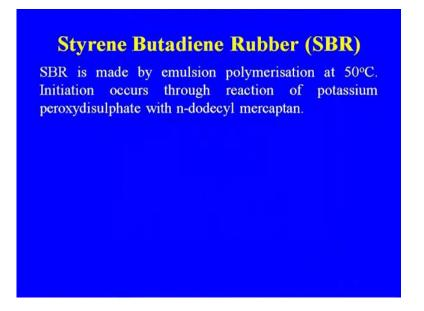
Rubber is made by emulsion polymerization at 50 degree centigrade initiation occurs through reaction of potassium peroxydisulphate with n-dodecyl mercaptan. Unit, so the chain propagation occurs by growing chain free radical of mercaptan attaching either butadiene or styrene. (Refer Slide Time: 17:21)
