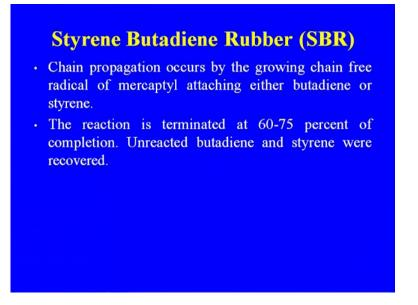
The reaction is terminated at around 60 to 75 percent of the completion of the reaction unreacted butadiene and the styrene are recovered.
