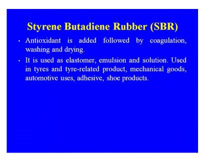
So, other actually additives are also added antioxidant is added followed by coagulation washing and the drying. It is used as elastomer emulsion and solution used in the tires tyre related product mechanical goods, automotive use, adhesive and the shoe products another important ethic under the polystyrene butadiene.
