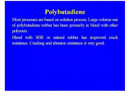
Blend with S B R or natural rubber has improved the crack resistance cracking and abrasion resistance is very good in case of the polybutadiene. It is characterized with a high abrasion and crack resistance better resistance to heat degradation and the blowouts, good hysteresis properties, large scale use in the tyre cord modification of the plastic conveyor.
