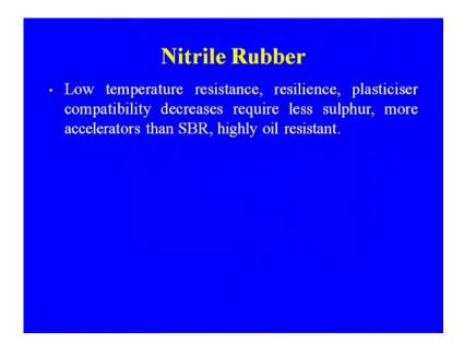
These are the some of the characteristic of the nitrile rubber application fuel hoses collapsible containers nitrile rubber may be reinforced by phenolic resins and P V C.
