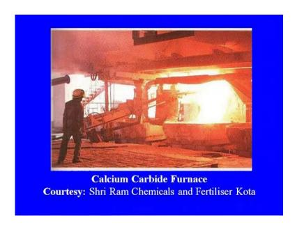
This is the calcium carbide plant; you can see that the environmental condition of plant this is the route, and how we are making the calcium carbide.
