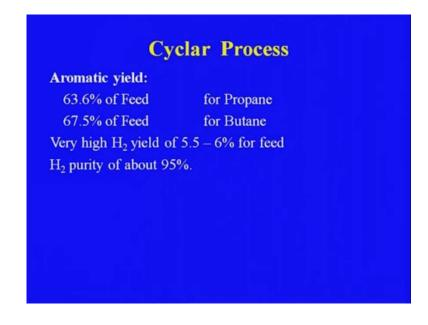
So, feed is propane and butane, pentanes or mixtures of these. Liquid product largely BTX essentially free from C6, C9 paraffinic and naphthalenes. So, this is more pure from other that we are getting. Preparation of benzene, toluene and xylene charges are very little with the composition of the feed.
