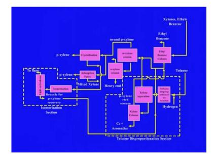
This is the process we are using in case of the separation because this is the again what about your after the separation of the toluene and ethyl benzene. Mix xylene that we are getting containing the ortho xylene para-xylene and meta-xylene. And the xylene or meta and para they are having the close boiling point. So, they cannot be separated by the distillation. But, ortho xylene which is having around 140 degree centigrade boiling point so that is separated by distillation here.
