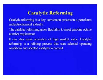
Now, let us discuss very brief about the catalytic reforming which we discussed in detail in the model 6; that the catalytic reforming is the key conversion process in the petroleum petrochemical industry. From the petrochemical point of view it is important for the protection of the aromatics in the hydrogen that we are getting as a bi-product and from the reformative you can separate this aromatic.
