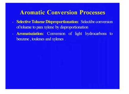
So, how to utilize this effectively to increase the productivity or the reduce the cost of the para-xylene manufacture? That will be the isomerisation or the toluene disproportionate that may be there. Aromataziation that is the conversion of the light hydrocarbon comes to benzene, toluenes and xylene similar to your reforming process.
