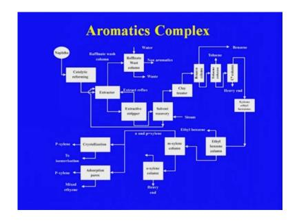
This is the typical aromatic complex where the combination of the catalytic reforming and the separation will be discussing separately. Then, it will be more clear where we are having the extractive discussion for the separation of a aromatics from the non aromatics then, the clay treatment and then, the various distinction column where, separating the benzene which is the lower boiling point toluene and xylene mixture that will we can.
