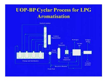
This is the typical LPG aromatization you need to develop by UOP and where again, we are again having the series of the reactors and this is the stack inter heaters and this is the
