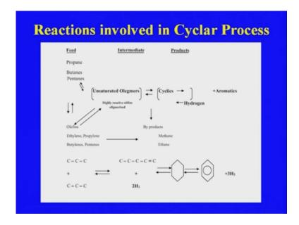
So, this was the cycler process that is being used for the, these are the some of the series of the reaction that is taking place from the in the cycler process where you getting the hydrogen which I told you the high hydrogen and this is the aromatics that you are getting. So, these are the series of the reaction that is taking place in the process of the conversion of the natural gas to the or propane butane to aromatics.
