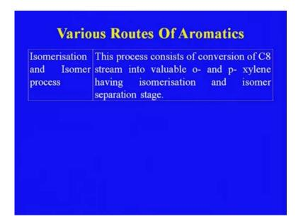
This process consists of the conversion of C8 stream into valuable ortho and para-xylene having isomerisation and the isomer separation stage. These are the two stages revolved in case of the isomerisation in it.
