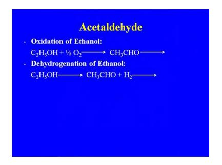
This is the process that is taking place, while the reaction that the oxidation of ethanol or the dehydrogenation of the ethanol.
