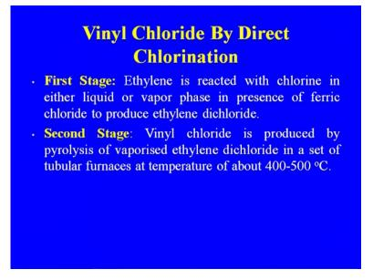
So, if you see the reaction in case of the these two reaction, di direct chlorination and oxychlorination. Here again, in case of the oxic here, HCL is also formed but here, in case of the oxychlorination, this HCL, whatever the HCL, that is consume in the
