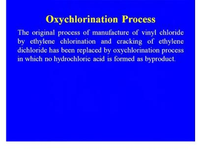
The original process of manufacture of vinyl chloride by ethylene chlorination and cracking of ethylene dichloride has been replaced by oxy chlorination process. In which, no hydrochloric acid form as a byproduct, which was a problem in case of the direct chlorination process already we have, I discussed that point.
