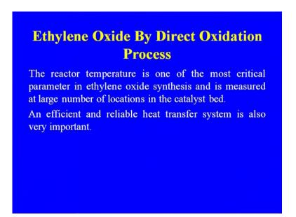
So, the reactor temperature is one of the most critical parameter in ethylene oxide synthesis and is measured at large number of locations in the catalyst bed. Because temperature that is playing a very important role here. Because you will have to suppress the side reaction, which is taking place and efficient and reliable heat transfer system is also very important.
