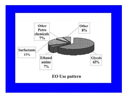
These are how the ethylene oxide used pattern, that the major portion you see the ethylene glycol ethylene glycol. Because during the process as I told you the, all the three are formed but you can optimize the condition of the from... So, that the higher
