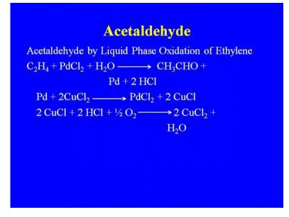
This is the reaction that is taking place in case of the liquid phase, again the palladium catalyst that we are using.
