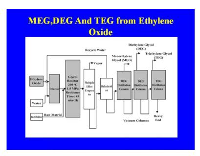
This is the process flow diagram for MEG and here, if you see the ethylene oxide then the water, inhibitor, that is going to the dilution. After dilution, it is going to the glycol rector, this is the temperature, (( )) your pressure condition residence time is about, this is the residence time. And then the this is the actually the multiple effective operator and during the process because here, you will have to control the ethylene oxide to water ratio to maximize the yield of the MEG.
