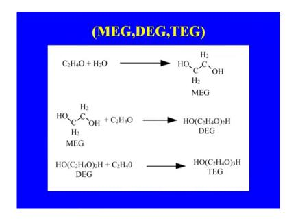
This is the reaction that is taking place during the manufacture of the ethylene glycol from the ethylene oxide and the here, you see the various reaction that is taking place MEG, DEG, TEG. So, this is the how the, why the we are controlling the ratio of the ethylene oxide to water, to have the maximum MEG.
