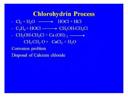
This is the reaction that is taking place in case of the chlorohydrin process and the chlorohydrin that is going for the manufacture of ethylene dioxide. So, corrosion problem, one another byproduct you can say, the waste you are generating that the calcium chloride. So, these are the two major problems, which relate to the use of the oxidation process of the chlorine ethylene sorry not chlorine, ethylene.
