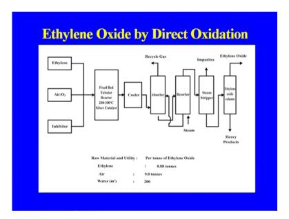
So, this is the process, we are having the flow diagram for making of the ethylene oxide, ethylene air inhibitor, that is going to the fix bed. Tubular reactor where, the temperature you know around 200 to 300 degree centigrade cooler than absorber, as I told you the CO
