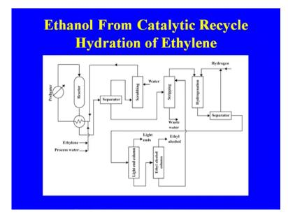
So, this is the process we are using in case of the ethanol by hydration by vapor phase hydration of the ethylene that you are getting the ethanol. This is the process, that we are using for from the using the ethylene for making of the ethanol. Now, let us discuss one of the very important product of the ethylene that is, the acetaldehyde.
