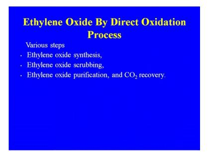
Ethylene oxide by direct oxidation process, various steps involve in case of the ethylene oxide ethylene by oxidation process, ethylene oxide synthesis, ethylene oxide scrubbing.
