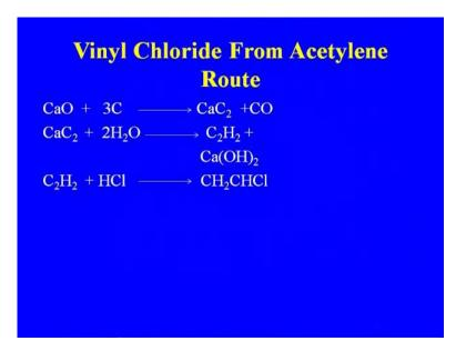
So, this was the actually, they are real route for making and this is the reaction we are getting the acetylene and acetylene after the chlorination, that the that is here then then it will go to for the formation of the vinyl chloride. So, direct chlorination process where, we are using, no this is not the, we are not using the oxygen.
