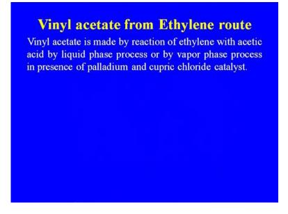
So, vinyl acetate is made by reaction of ethylene with acetic acid by liquid phase process or by vapor phase process in presence of the palladium and cupric chloride catalyst. This is the process, which now being used for the, even the the units which are making the vinyl acetate from the ethylene, from molasses route alcohol to ethylene so they are using this process.
