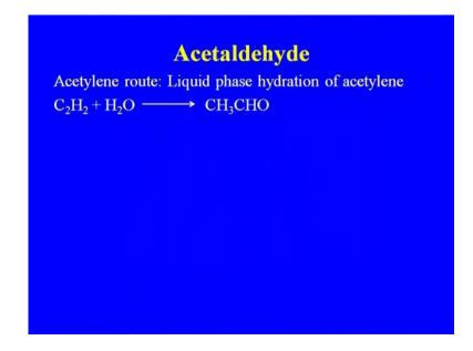
This is the acetylene route liquid phase hydration of the acetylene where, you are getting the acetaldehyde, this process is no more it has been used.
