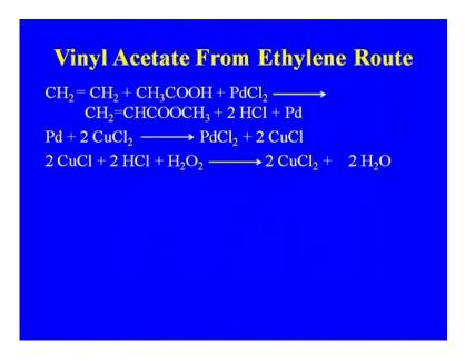
These are the reaction series of reaction that is taking place and the catalyst, which are using palladium catalyst.
