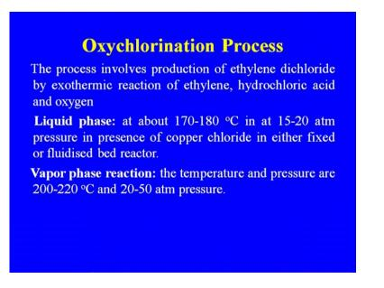
In case of the oxy chlorination process, the process involves production of ethylene dichloride by exothermic reaction of ethylene, hydrochloric acid and oxygen. Because here the what about the hydrochloric acid is produce in the process that is being utilize.
