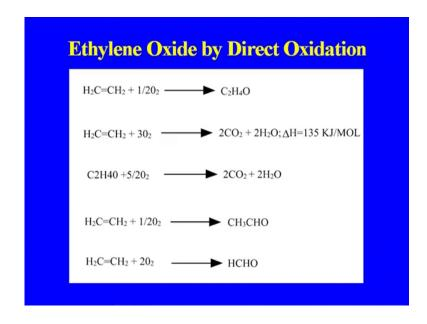
This is the reaction that is taking place and in the reaction, if you see that the we are also getting some of the side reaction also there. Undesirable side reaction, which are not unavoidable, this the CO 2 formation, huge amount of the CO 2 that is formed there in the process and so that has to be removed continuously.
