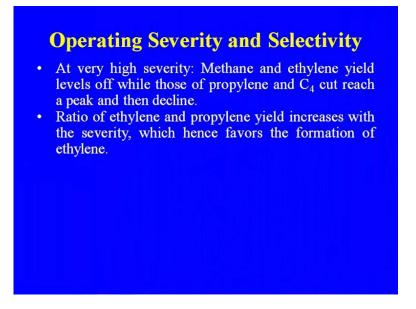
At very high severity methane and ethylene yield levels off while those of propylene and C 4 cut reach a peak. Then decline ratio of the ethylene and propylene yield increases with the severity, which hence favors the formation of the ethylene.
