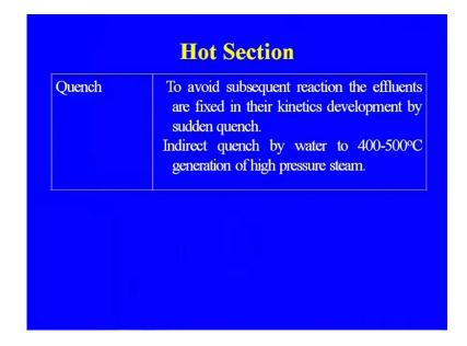
So, to avoid this subsequent reaction the effluents are fixed in their kinetics development. By sudden quench indirect quench by water to 400-500 centigrade and which we are using for the steam. We are generating that is using the system so this is the indirect quench that we are doing in case of the cracking plant. Because that is important quenching because the transfer line what will happen if the more and more coke formation is there than the run length.
