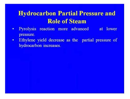
Role of the steam which I was telling that why we are using steam due to say that overall reaction rate enhance the selectivity of pyrolysis on favor of the light olefins, which I desired and increases the temperature of the feed stock. So, that they also helping in the increasing the temperature before it is going to the cracker.
