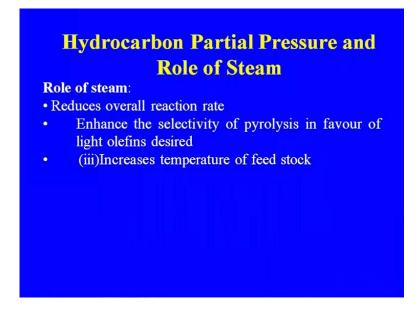
As I told you the 1 term very important term that we are using incase of the furnaces that the operating severity and selectivity, because this, what we need incase of the cracking that the more and more lighter product then the heavier product.
