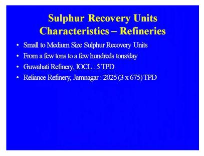
Sulphur recovery units characteristics small to medium size sulphur recovery units and from a few tons to a few 100 tons per day Guwahati refining, because of the sulphur content is low, the sulphur production is less. But, in case of the Reliance Jamnagar processing where they are processing more heavier fluid stock production of the sulphur is high.
