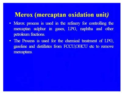
Merox process is used in the refinery for controlling the mercaptan sulphur in gases LPG, naphtha and other petroleum fraction. The process is used for the chemical
