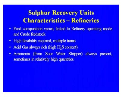
Sulphur recovery units, feed composition varies linked to refinery operating mode and crude feedbacks. High flexibility is required, multiple trains, acid gas always rich high
