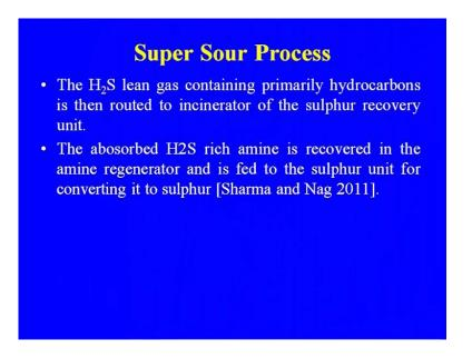
The H2S lean gas containing primarily hydrocarbons is then routed to incinerator of the sulphur recovery unit. The absorbed H2S regenerator amine is recovered and is fed to the
