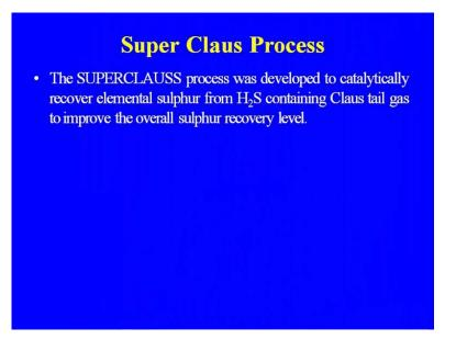
So, the super claus process was developed to catalycally recover elemental sulphur from H2S containing claus tail gas to improve the overall sulphur recovery level in the diefining.
