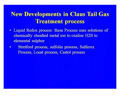
This is another process that we are using which we are liquid redox process: uses solutions of chemically chealted metal ion oxidize H2S to elemental sulphur. So, these are some of commercial process which are available for stretford process, sulfolin process, sulferox process, locat process, castol process. These are the some of the process that is available to meet the required standards the chemical process.
