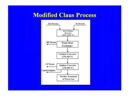
This is the modified claus process here you see the H2S that is the stream term director oxygen is stream. It is going to waste heat boiler, catalytic converter, sulphur condenser. From where we are getting sulphur and further treatment of the waste gas that is so, the modified claus process. So, what are the various typical of the super claus process?
