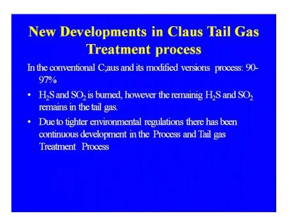
New development in claus tail gas treatment process in the conventional claus and its modified versions process 90 to 97 percent, because 90 to 97 percent that is on the hard side depending upon the efficiency of the claus process. The emission the conversion that may be as low as 90 percent H2S and SO2 is burned, however the remaining H2S
