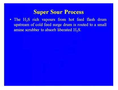
In case of the super sour process the H2S vapors from hot feed flash drum upstream of cold feed surge drum is routed to a small amine scrubber to absorb the liberated H2S. So, that is the telling at the additional, which I feature of the super sour process that is going to the amine from the recovered from this part. So, that is going amine discovered and the weightier involved efficiency there.
