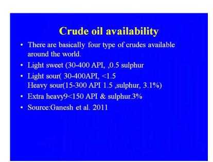
There are basically four types of crudes available around the world that already we have discussed that we are having the light sweet and light sour, heavy sour, extra heavy sulphur. So, this is how that sulphur content that is varying, gravity that is varying or in case of light that is 30 to 40 light sour. But in case of the heavy sour it is more heavier
