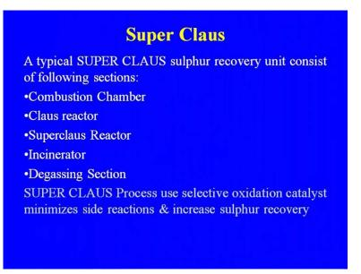
Combustion chamber, claus reactor, super claus reactor, incinerator, degassing section. Super cluas process use selective oxidation catalyst minimizes side reactions and increase sulphur recovery.
