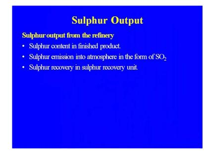
So, the sulphur content in finished product sulphur emission into atmosphere in form of SO2. This is coming to the because we are speaking about the sulphur output from the refinery. Sulphur recovery- in sulphur recovery unit there are nearly the clause process or modify process been up to 97percent. Some of the sulphuric compound is still remaining, so because of that reason now we are going for the has been development in the sulphuric units to achieve maximum sulphur compound.
