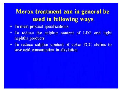
Merox treatment can in general be used to meet the product specifications to reduce the sulphur content of the cooker FCC, olefins to save acid consumption in alkylation process.
