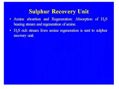
So, amine absorption and regeneration, it is the process which I told you absorption of the H2S, where H2S is bearing stream, and regeneration of amine. H2S rich from amine regeneration is sent to sulphur recovery unit for recovery of the sulphur from the gas. Now, let us discuss the merox process, that is the integral part of the refinery, and all the refinery they are having merox process.
