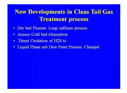
So, these are the some of the process developed for the treatment process is dry bed process, Lurgi sulfreen process, amoco cold absorption, direct oxidation of H2S, liquid phase sub dew point process: that is clauspol process.
