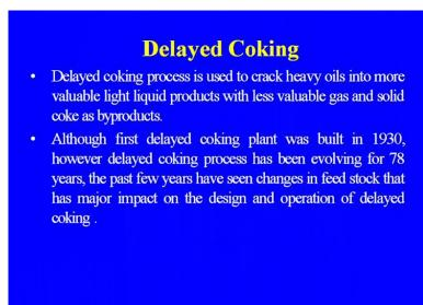
Now, let us discuss in more detail about the delayed coking. Delayed coking process is used to crack heavy oils into more valuable light liquid products with less valuable gas and solid coke as by products. Although the first delayed coking plant was built in 1930, however delayed coking process has been evolving for the last 70 80 years, the past few years have been changes in feed stock and has major impact on the design and operation of the delayed coking.
