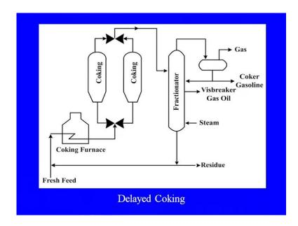
This is about the delayed coking, here the feed is going to the coking furnace a temperature is raise here and then it is going to the coking drum and from the coking drums it is going to the fractionators, again from the fractionator we are getting the different product the gas, coker gasoline that may be there, coker gas oil we are getting and the residue from the fractionator and from the coking process, so that will be the residue that will be getting.
