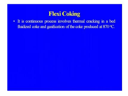
It is continuous process which involves the thermal cracking in a bed fluidized coke and gasification of the coke produced at 870 degree centigrade. So, this is the flexi coking.
