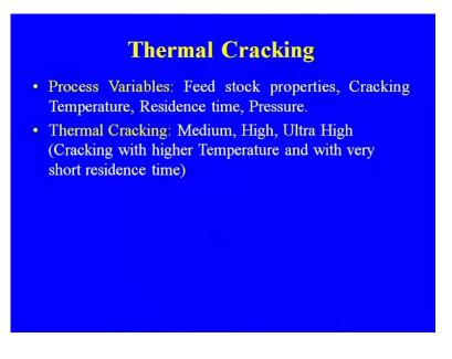
Thermal cracking that may be medium, high, ultra cracking with ultra high cracking means the cracking with higher temperature with very short residence time, because the residence time that is playing very important role in the cracking processes in the formation of the coke.
