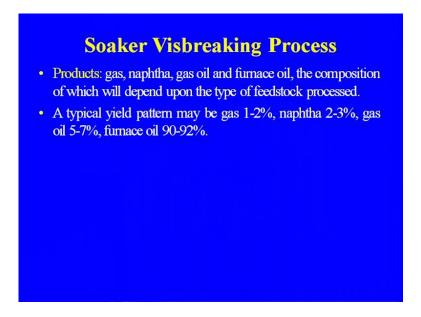
Soaker vis breaking process; the products which we are getting from this are gas, naphtha, gas oil and furnace oil the composition which will depend upon the type of the feed stock process, which I told you depending upon the feed stock the whole product range which we are getting about the cracking that will vary. A typical yield pattern may be gas 1 to 2 percent, naphtha 2 to 3 percent, gas oil 5 to 7 percent, furnace oil that is 90 to 92 percent.
