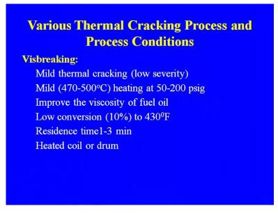
Now, let us discuss some of the important thermal cracking processes and the process condition then we will go in detail about the individual process. This is the condition we are using in case of the vis breaking, mild thermal cracking, low severity, temperature is 470 to 500 centigrade at 50 to 200 P S I G, improve the viscosity of the fuel oil, low conversion residence time 1 to 3 minute heated coil or drum that we are using.
