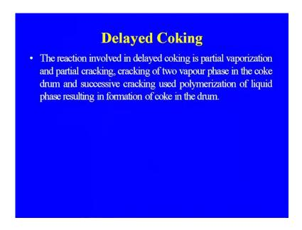
The reaction involved in delayed coking is partially vaporization and partial cracking, cracking of two vapour phase in the coke drum and successive cracking used polymerization of liquid phase resulting in the formation, because always the formation of the coke is because of the polymerization reaction that is taking place in any furnace or any process.
