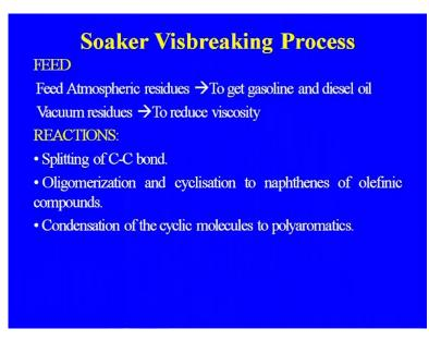
Feed to the soaker or atmospheric residue to get gasoline and diesel oil vacuum residue to reduce the viscosity. So, depending upon the feed which we are using in case of the visbreaker, the type of the product which is getting that will vary. Reaction; these are the reaction, already we have discussed everything oligomerization and cyclisation of the naphthenes condensation of the cyclic molecules. So, the different reactions are taking place.
