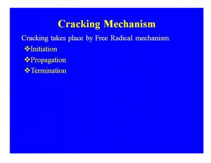
So, the cracking mechanism, so whatever the cracking reaction that is taking place as the free radical mechanism, initiation, propagation and the termination. So, these are the steps that are taking place during the cracking process.
