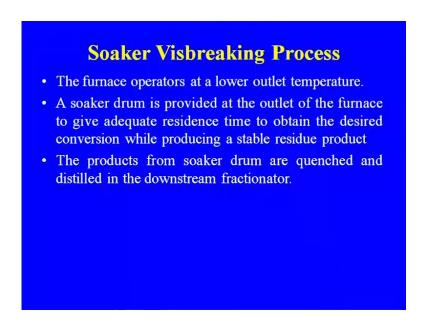
Soaker vis breaking process, the furnace operates at a lower outlet temperature. A soaker drum is provided at the outlet of the furnace to give adequate residence time to obtain the desired conversion while producing a stable residue product. The products from the soaker drum are quenched and distilled in the downstream fractionators.
