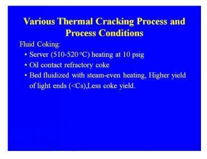
Fluid coking we are having the severe higher temperature severe condition and so 500 to 520 oil content and the refractory coke, fluidized bed we are using with steam even heating higher yield of the light ends less coke yield is there in this process. Let, us now discuss the vis breaking process, the detail of the vis breaking, because this is one of the important unit in refinery as I told you earlier also.
