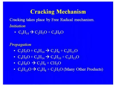
Initiation, this is the reaction that is taking place in the initiation and the lighter product we are getting and again from the propagation, this is converted too much other large number of the product, finally the termination where we are getting some of the lower molecular weight hydro carbons.
