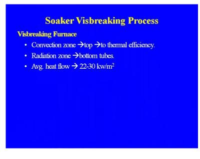
Vis breaking furnace in the furnace we are having the convection zone that is top to thermal to increase the thermal efficiency radiation zone, bottom tubes where actually the cracking is taking place, average heat flow this is for a particular case, 22 to 30 kilo watt per meter square.
