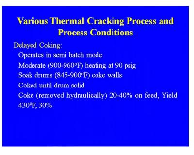
Delayed coking operates in semi batch mode, moderate temperature heating at 90 P S I G, soak drums are used coked until drum solid that is separated, there coke removed
