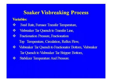
Variables, in case of the soaker vis breaking process, what are the variables? Feed rate, furnace transfer temperature, visbreaker tar quench to transfer line, fractionation pressure, fractionation top temperature, circulation, reflux flow, visbreaker tar quench to
