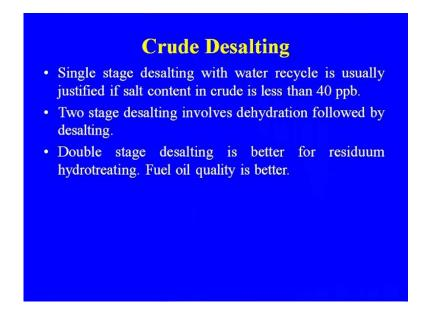
So, this is about the single stage desalting with the water recycle usually justified if the salt content in the crude is less than 40 ppb. If the low salt content is there two stage desalting involve dehydration followed by desalting. Double stage desalting is better for residuum hydro treating fuel oil quality is better, so this is the reason why the we are having the two stage desalting process.
