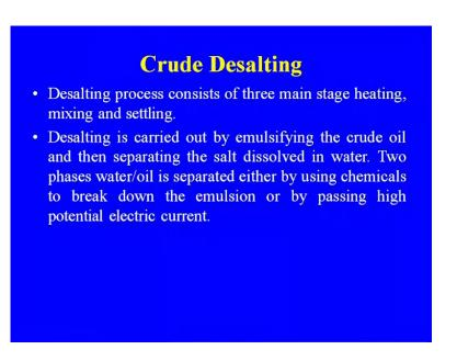
So, what are these this is involved in case of the desalting? Desalting process consists of three main stages; heating because a particular temperature low or high temperature that is affecting the if you sea of the desalting process. So, heating of the crude oil mixing and settling because the separation of the impurities, which has there after the, because
