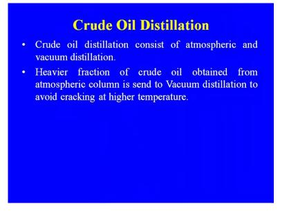
So, crude oil distillation consists of the atmospheric and the vacuum column vacuum distillation, why we are going for the vacuum? We know that under vacuum the lower temperature that will be required otherwise the higher temperature. Then the cracking reaction that may take place so, that is why the atmospheric in vacuum distillation both we are using and that is the integral part of any refinery.
