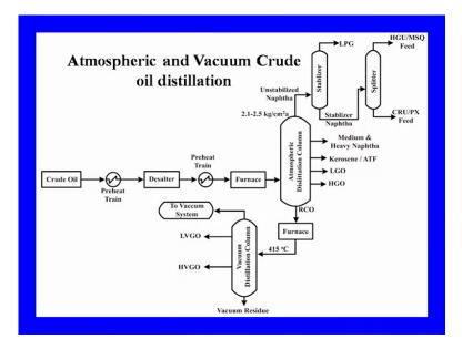
So, the atmospheric column, what is happening? The preheated desalted crude that will go to the pre flash section distillation column and the stabilization of the naphtha because the naphtha, which we are getting especially the lighter component of the naphtha, the gases has to be removed from the light gases LPG. That has to be removed from the light naphtha and the light naphtha again it will go through as we what we call it the styrene gasoline, which will go to the gasoline form.
