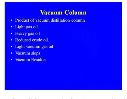
These are the products, which we are getting from the vacuum column light gas oil, heavy gas oil, reduced crude oil, light vacuum gas oil, vacuum slops, vacuum residue. Light gas oil that is the feed for the FC and now the with the coming of the hydro cracker we are also able to part process the heavy gas oil, fraction or it may light or the heavy that may go to the RFC or it may go to the hydro cracker units.
