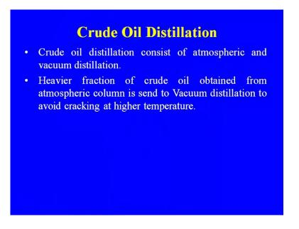
Heavier fraction of the crude oil obtained from the atmospheric column is send to the vacuum distillation column to avoid the cracking at higher temperature. Let the
