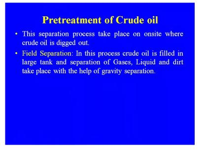
The separation takes place onsite where crude oil is digged out as tiding at this field separation. In this process crude oil is filled in large tank and separation of the gas liquids and dirt takes place with the help of the gravity separation. So, the some of the impurities that we are removing even the pretreatment for the removal of the eminent treatment also we are doing for the removal of the sulfur compounds.
