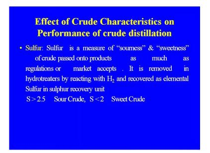
Sulfur is the measure of the sourness and the sweetness of the crude passed onto the products because, this is the one of the actually they compound which is causing corrosion problem in the process. So, it is removed in the hydro treaters by reacting with the hydrogen and recovered as an elemental sulfur, but the some of the removal if the more that will create the corrosion problem.
