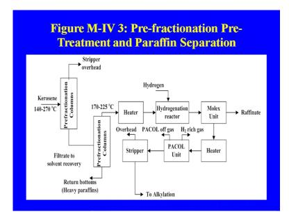
Pre-fractionation column then the stripper overhead again filtrates to solvent recovery, this is going to the, this is not part of this, this is coming in the other. So, prefractionation column and then the finally, the return bottom to the heavy paraffins that will be jumped to this, and that will be used a fuel again and so, it will go to the heater hydrogenation reactor hydro treatment means, the pre treatment of the paraffins, which we are separating from the fractionation column.
