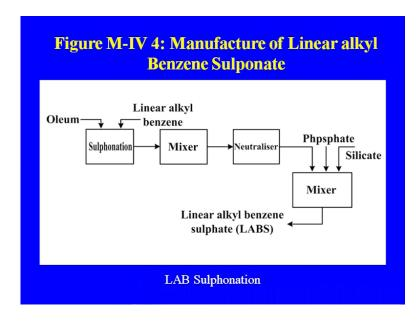
This is the process which I discussed earlier the linear alkyl benzene sulphate, where the you are doing the sulfonation mixture, neutralizer and then silicate phosphate as a filter. And other ingredients of the surfactant that we are and the final, you will be getting the L A B. Again the final formulation of the detergent, which you are getting the finished product, because this is the basic raw material that has been supplying by the LAB
