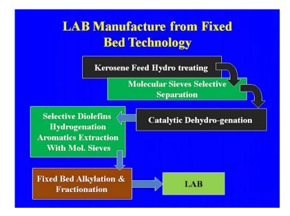
So, here again as in the case of the HF catalyst the process, which we discussed kerosene feed hydro treating after the fractionation because here, this is only the simplifies flow diagram with that will have to fractionate. The kerosene we will have to get the paraffin
