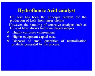
So, HF acid has been the principal catalyst for the production of LAB from the linear olefins, and most of the plans before coming of the Indian oil plant at Vadodara in India. All the plant there are based on the H F's hydro fluoric. How about the handling of the corrosive catalyst such as hydrofluoric acid? They have always some disadvantage, that I told you the corrosiveness, and from the environmental norm highly corrosive
