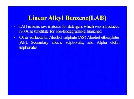
Other surfactants are also there that is getting important that the alcohol sulphate alcohol ethoxylates, which I was telling about the ethoxylate secondary alkane sulfonate and alpha olefin sulfonate, these are also being use in the detergent industry because these are the some of the alternative raw materials also.
