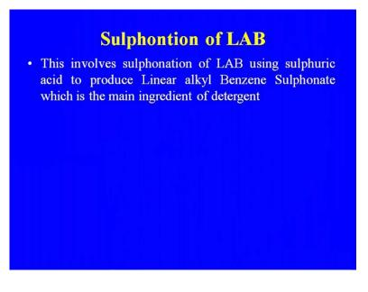
This involves using sulfuric acid to produce linear alkyl benzene sulfonate, which is the main ingredient that of the detergent.
