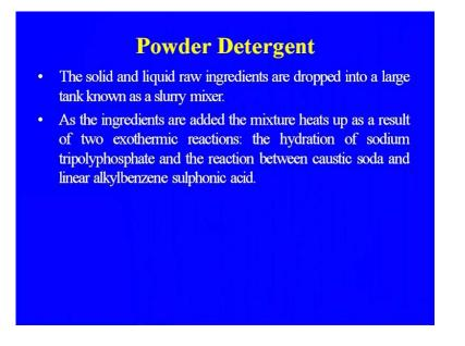
The solid and liquid raw ingredient drop into a large tank known as a slurry mixer, and as the ingredients are added the mixture heats up. As a result of the two exothermic reactions, the hydration of the sodium tri-phosphate and the reaction between caustic soda and the alkyl benzene sulphonic acid.
