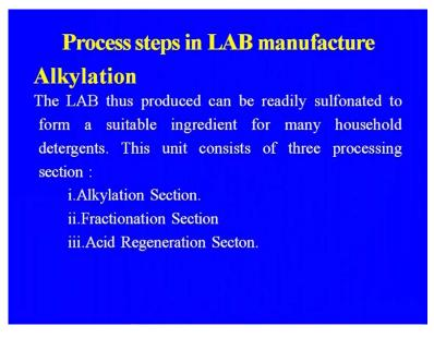
So, the next in case of the LAB thus produced can be readily sulfonated to form a suitable ingredient for many a household detergents. This unit consist of alkylation because the product of the alkylation that you have the alkylation section, fractionation section, acid regeneration section because the acid recovery that is very important if you are using the hydrofluoric acid.
