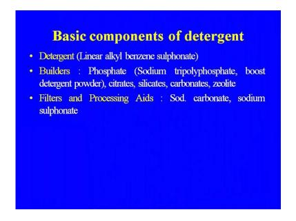
Basic component of the detergent you see, the detergent that is the base is the linear alkyl benzene sulfonate because most of the detergent all the detergent. They are now, using the linear alkyl benzene sulfonate builders, phosphate sodium tripolyphosphate and boost detergent powder, citrates, silicates, carbonates, zeolite these are the builders filters and processing aids sodium carbonate and sodium sulfonate that we are using.
