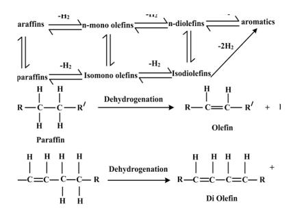
This is the reaction that is taking place in case of the pacol process. Now, the next step as I told you in case of the after making of the linear alkyl benzene, this is the sulfonation of the linear alkyl benzene.
