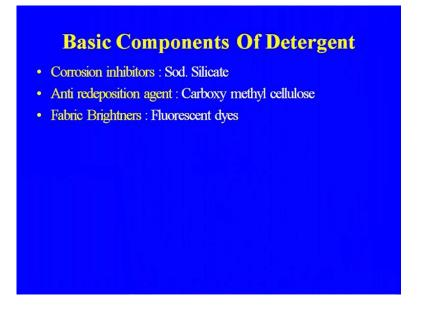
Corrosion inhibitors that it also either it has sodium silicate, anti re deposition C M C methyl cellulose that was fabric brighteners fluorescent dyes that we are using, in case of the fabric brighteners.
