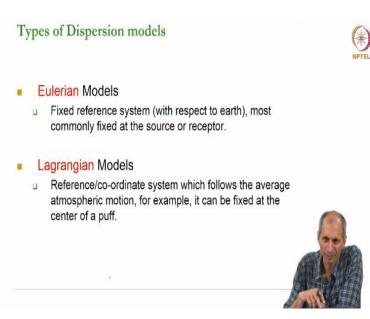
So dispersion models can be of two different kinds. So, one what is called as an Eulerian model, which is fixed reference frame. So what this means is that I am modeling this room here. I have watching from here. So x equals 0 begins at that end goes to this end start from here and here. Lagrangian model on the other hand is that you are moving with the fluid and your frame of reference is that body of fluid.
