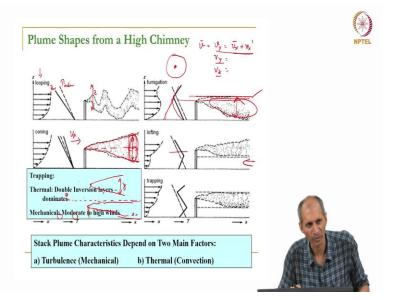
So we have different types of plume shapes that it can take. And the 2 main factors here so here we will go over each one of them. The first one is called as looping the super adiabatic lapse rate, which means that the lapse rate is greater than the this slope of this line - DT by DZ is greater than this one. No super adiabatic means the environmental lapse rate is greater than this. That is only because this one does not change adiabatic lapse rate stays where it is the other thing changes.
