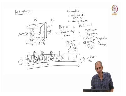
And this this concept is known as a box model. And we will come back to this river system in a minute. We call what is a box model a box model, essentially is it is a box is a 3 dimensional box. It has a certain volume is called it as delta x, delta y and delta z and in this volume, there is a concentration rho A2, rho A1 whatever we call it rho A2 for the time being. The basic assumptions of the box model is that this well mixed the contents are well mixed.
