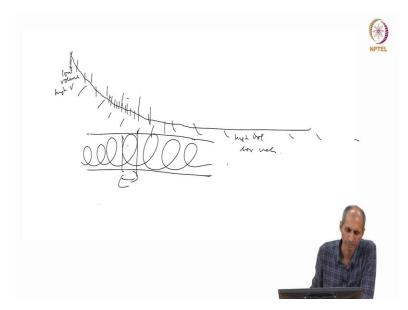
The river Ganges comes from somewhere in the in the hills, his gradient is like this and then as it comes down to the upper plains and then lower plains it becomes like this. Here the velocity is very high, until it comes here the volume is low here, velocity is high here. Low volume, high velocity here high volume, the lower velocity, the terrain, the nature of the bed of the river is very different in the upper reaches and as we come down into the plains becomes very different.
