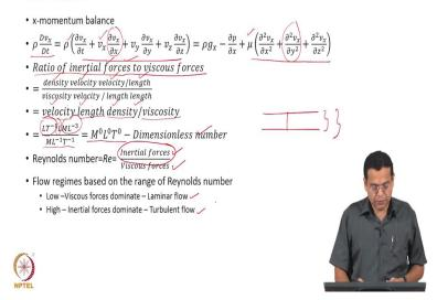
Now, the flow regime tells about characteristics of a flow and different regimes will have different characteristics and they depend on the velocity of the fluid, the properties of the fluid and the geometry as well. Now, we need to discuss about this flow regime now because that will tell the scope of the present discussion namely inviscid flows.
