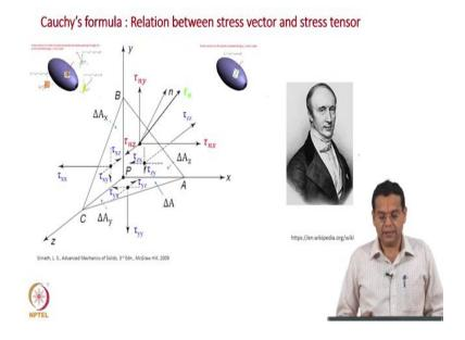
Then, we related these two the stress vector to the components of stress tensor using the Cauchy's formula.
