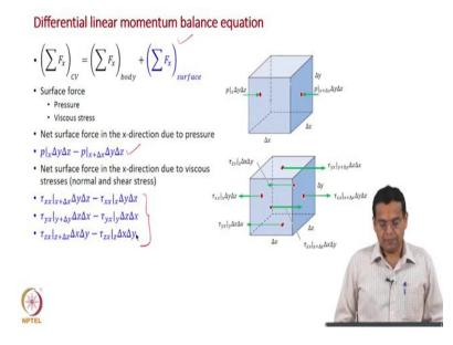
So, now our attention was on the surface forces, specific attention was on the surface forces, we express the surface force for pressure and for the viscous stress.
