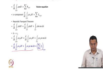
We applied the Reynolds transport theorem. So, the left hand side was expressed in terms of a transient term and a convection term for the control volume, right hand side was still in terms of system we took a coincident system and control volume. So, right hand side became that for the control volume. And, that is the integral form of linear momentum balance equation.
