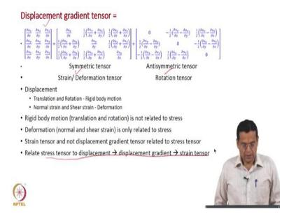
And, more importantly we discussed that the displacement gradient tensor a sum of strain tensor and rotation tensor. And, we also said that the stress tensor has to be related to the strain tensor. Now, at that point we have completed these two blocks. We will have to extend that knowledge analogues to fluids, where we discuss the strain rate and strain rate tensor.
