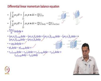
And, then we combined with our earlier transient term convection term and the gravity on the right hand side, along with that we included the surface forces due to pressure and viscous stresses represented by all this 4 I would say control volumes.
