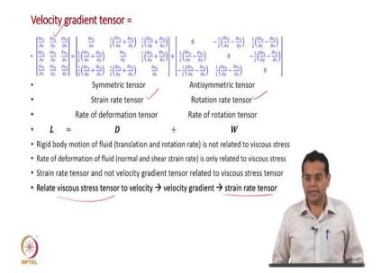
And, once again more importantly we discussed, the velocity gradient tensor a sum of a strain rate tensor and rotation rate tensor. Once again we said the objective is to relate viscous stress tensor to the strain rate tensor.
