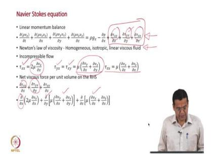
So, let us do that. The starting point is the linear momentum balance equation. So, our starting point is the linear momentum balance equation of course, there are 3 equations one for each direction, let us write down the equation for the x direction.
