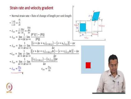
And, we discussed normal strain rate and shear strain rate, we said they are material derivatives of normal strain and shear strain, and then we related the normal strain rate to velocity gradient, shear strain rate to velocity gradient
