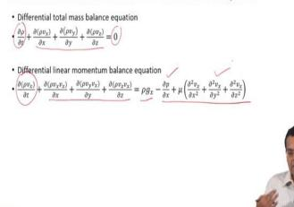
And, now we can compare the differential total mass balance and the linear momentum balance equation,
