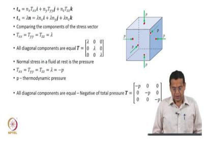
So, we got the component of total stress tensor under hydrostatic condition.
