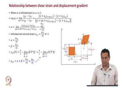
The normal strain in terms of displacement gradient, the shear strain in terms of displacement gradients.
