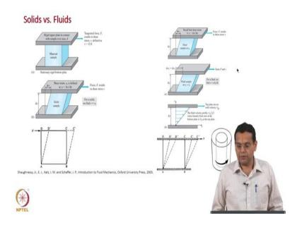
Few slides from there, we have once again discuss the difference between solids and fluids to understand that it is strain for solids and strain rate for fluids. Force depends on stain for solids and force depends on strain rate for fluids.
