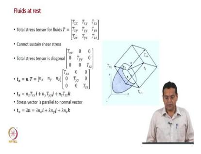
Based on that, we discussed the stress in a fluid under static condition, which is normal stress, which is pressure the thermodynamic pressure and is compressive hence -p.
