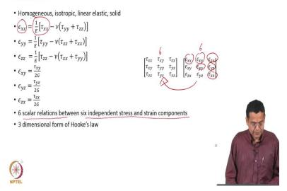
Those are the stress tensor and the strain tensor. So, those are the assumptions which have discussed homogeneous, isotropic, linear, elastic, solid. We can now summarize all the relationships which have discussed so far for normal strain and shear strain. So, we have seen as the expression for normal strain along x axis, analogously we can write an expression for normal strain along y axis; similarly normal strain along z axis.
