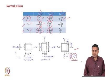
Now, based on this let us come discuss this table. What this table shows us that the column headings are the normal stresses along x direction, y direction, z direction. What are the row headings? The normal strain along x direction, y direction and z direction.
