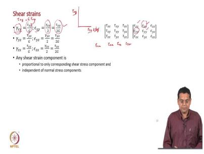
So, for we have discussed about normal strain. So, now, let us discuss about shear strain. We introduced the shear modulus based on the linear relationship between  $\tau_{xy}$  and  $\gamma_{xy}$ . We said  $\tau_{xy}$  versus  $\gamma_{xy}$  is linear and the proportionality constant is shear modulus.
