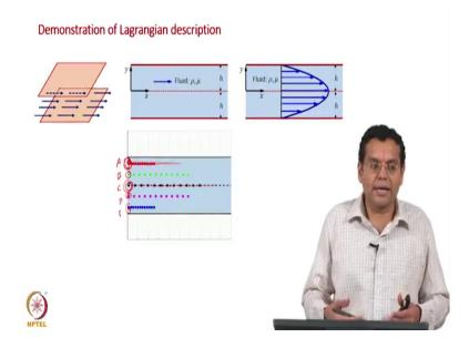
So, first to demonstrations to represent the Lagrangian description, Eulerian description. Think the geometry and the plates are same as I discussed earlier, flow between two parallel plates. Now, let us straight away run this simulation ok. What we say Lagrangian description is identifying a fluid particle and tracking it, and that is what has been done here. We have identified a fluid particle, and then we are tracking that as it flows through the domain.
