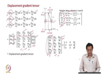
$\begin{bmatrix} du_x \ du_y \ du_z \end{bmatrix} = \begin{bmatrix} \frac{\partial u_x}{\partial x} \ \frac{\partial u_x}{\partial y} \ \frac{\partial u_x}{\partial z} \ \frac{\partial u_y}{\partial x} \ \frac{\partial u_y}{\partial y} \ \frac{\partial u_y}{\partial z} \ \frac{\partial u_z}{\partial z} \ \frac{\partial u_z}{\partial x} \ \frac{\partial u_z}{\partial z} \end{bmatrix} \begin{bmatrix} dx \ dy \ dz \end{bmatrix}$
