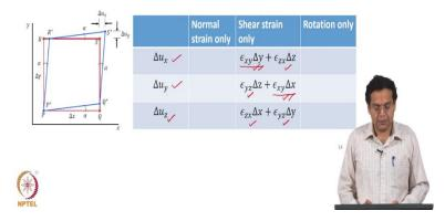
Just complete for other directions ok, this expression which we have written in the previous slide, difference in x displacement due to shear strain only, difference in y displacement due to shear strain only.
