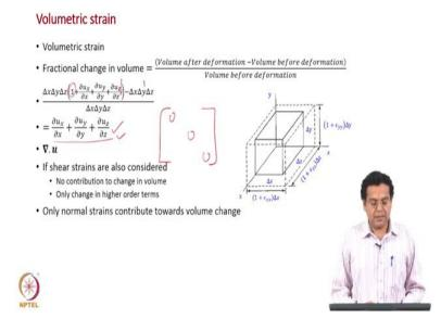
Now we can find out the expression for volumetric strain; volumetric strain how do you define?
