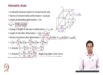
We have related normal strain, shear strain, rotation to the displacement gradients. Now we look at another strain which I have not defined we will define and also related to the displacement gradient that is called the volumetric strain. Just like the normal strain tells about change in length the shear strain tells about change in angle, rotation tells about rotation, volumetric strain tells about change in volume, in a 2D it will tell about change in area.
