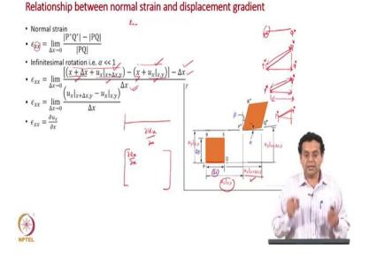
Now we are proceeding towards deriving a relationship between normal strain and displacement gradient. Now let us start with the definition of normal strain.
