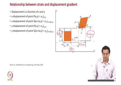
Moment you, let say type in your Google Strain Displacement Gradient this figure is the most popular figure you will come across, same figure has been taken from Ryman Parnes and let us understand this gradually. The x axis and y axis are shown and then you have plate PQRS is shown, in the initial state undeformed configuration. Now two ways of visualizing this; one is as I told you a plate, easy you to understand, other way should understand is it is a square region inside a solid object.
