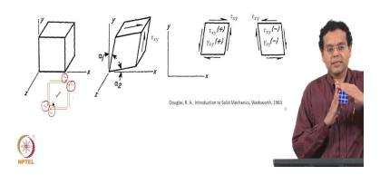
Take an object your shear stresses are the forces which will act in the opposite directions. It will make the object to shear in a particular way that is what is shown (in the above figure) which means the angle which has original 90 degrees will now decrease and we know that from the definition of a shear strain that the decrease in angle results in a positive shear strain. So, positive shear stress results in a positive shear strain. I will just repeat it.
