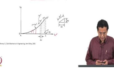
• A wire of finite length L, initially lying in the x-direction is stretched along a rigid track, which is a parabola  $y(x) = bx^2$ . All points of the wire displace in the y-direction only. Compute the strain at all points x of the wire.
