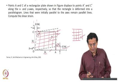
We will take an example for evaluation of the shear strain. Now, the what is shown here is a plate and you are given the un-deformed configuration you are given the deformed configuration, initial state and final state. Always remember, in all these cases a force is applied and it continued to apply and then it is it undergoes deformation.
