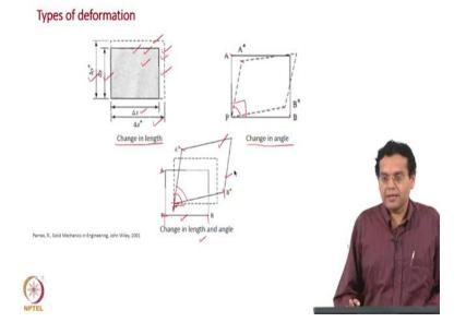
Let us start with types of deformation. How do you understand this visualizes? We take a plate and then let us says this is subjected to some force and because of the action of the force there is change in the dimension along x direction, change in the dimension along y direction. And so, the first type of deformation which can happen is change in length.
