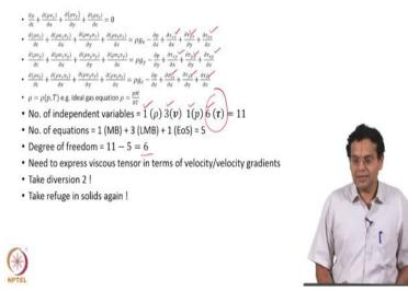
The equations are repeated here, we will do a degree of freedom analysis now for these set of partial differential equations. So, now, let us account for the number of variables number of equations; when I say variables I mean the dependent variables not the independent variables like time, x, y, z coordinates.
