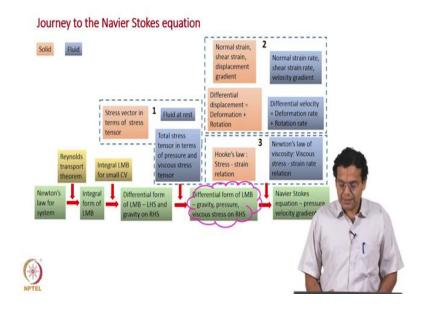
And, let me explain that with this journey to the Navier Stokes and where are we now and where are we proceeding. To begin with we started with Newton's second law of motion for system, applied the Reynolds transport theorem, derived the integral form of linear momentum balance, applied this for a small control volume, derived the differential form in the left hand side and the gravity on the right hand side.
