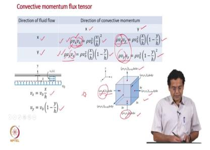
So, now convective momentum flux tensor, we have seen this earlier, what I have shown here are only 4 components of the 9 components because there are only two directions here. Two directions for fluid flow and two directions for the momentum, now as we have see in the previous slides the 4 components are
