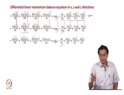
And of course, we can extend all this to all the three directions and that is what we will just write down here. All these three equations is going to come up along x, y and z directions together constitute the differential linear momentum balance equation though we are done for x direction, we can extend that to other three directions as well. So, let us complete.
