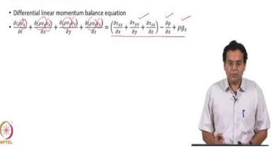
Just to compare the differential total mass balance and the linear momentum balance we will see how do they compare. So, that you know the similarity between the conservation equations that is the differential form of the total mass balance equation
