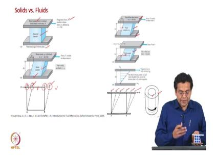
So, now we are going to discuss the difference between solids and fluids which will lead to our understanding of the total stress tensor. What I have shown on the left hand side, we have taken two plates and then let say we have a solid object.
