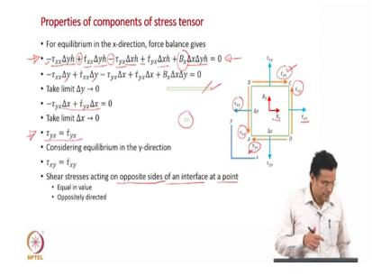
Now, we will discuss the properties of the components of stress tensor and how does it help us in terms of simplification. The two dimensional plane element is shown here. So, how do you imagine two ways of imagining, every kind of imagine is a plate like this or a character of imagining is the small two dimensional region inside a solid object as usual. We said tetrahedron inside a solid object now this two dimensional element inside the solid object.
