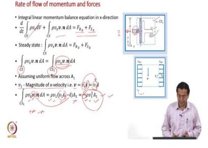
Let us write the integral linear momentum balance equation in the x-direction.
