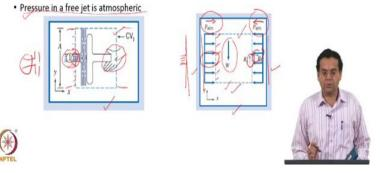
Now, the first step is to select the control volume and represent the forces. Now, the control volume that we have selected is shown here (left side image in above slide). When you look at the control volume, there is a momentum flow that crosses the control volume and then there is a force of our hand on the control volume which acts as the part of the control surface.
