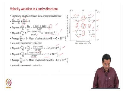
Now, we are going to use the continuity equation, once again we will assume it is a steady state and assume incompressible flow in the ocean and, remember it is a three dimensional case because we have all three components. We are going to apply this continuity equation at the point E.
