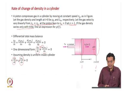
The last example as usual including the transient term, let us discuss the geometry first. I have a cylinder with the piston a well known geometry, let us say you would have come across in thermodynamics and mechanical engineering class etcetera. This could be a cylinder in an engine or reciprocating pump etcetera, of course, we are considering a gas here and we have a piston that moves at a constant velocity  $v_n$ .
