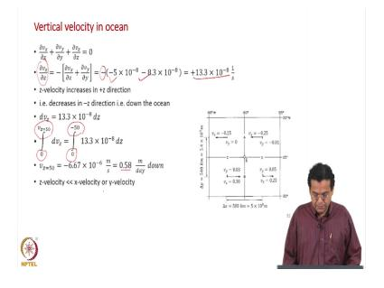
Now, let us substitute in the continuity equation to find out the  $\frac{\partial (v_z)}{\partial z}$ .
