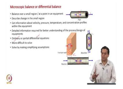
Now let us move on to the microscopic balance the differential balance. Now as the name indicates microscopic balance we take control volumes are within the equipment which are very small and in fact, every point is considered as a control volume.
