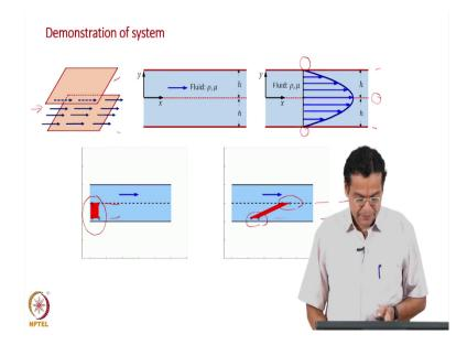
Let us take another example. This configuration is very well known to us just to quickly recap. We have two plates that are stationary and then fluid is made to flow through this using a pump. Then the velocity is 0 at the bottom plate; the velocity is 0 at the top plate, and it is maximum at the central line. So, what should we know, the velocity increases from the bottom plate to the central line, of course from top plate also it increases.
