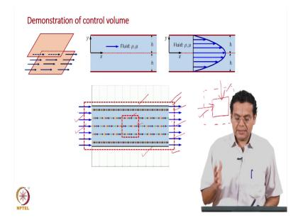
Let us demonstrate the control volume. The configuration fluid flow between the two plates is known to us. Now, let us straight go to the video (referee lecture video for visualization). Different fluid enters, and then crosses this region.
