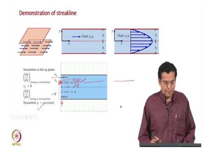
Now, let us have a demonstration for the streakline in the same geometry and same fluid flow conditions. So, let us straight away look at the demonstration of streakline. The way in which you have done is or what you have to focus is, here the simulation is run (watch video for better understanding) such that as if I am injecting a dye here, remember the prescribed point can change. If you want to get an entire flow field, you will have to change the point of injection.
