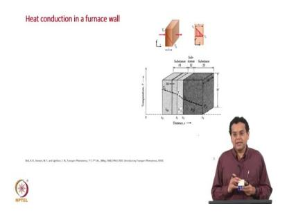
So, now let us extend the discussion what they had for a singles slab to a series of labs. What is an application? This can be taken as an example for a series of slabs. The application would be in a for a furnace wall, furnace is an equipment where we have very high temperature inside and we use it for carrying out high temperature reactions.
