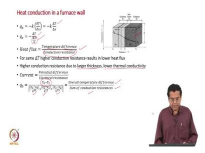
For that let is write the Fourier's law of heat conduction in terms of difference. So,
