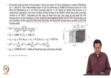
Let us take a numerical example to illustrate the theory which are discussed now for heat conduction of furnace wall. Let us read the example the furnace wall consists of three layers, the inner layer of 10 cm thickness is made of firebrick is thermal conductivities 1 W/m. K.
