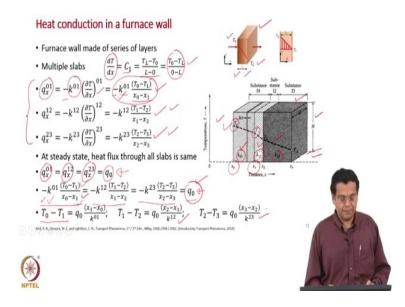
So, as I told you furnace wall made of series of layers or series of slabs, so we discuss in terms of multiple slabs. We will use a this result which you have seen in the case of single slab that is the temperature gradient or the slope of the temperature profile
