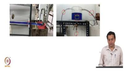
So, as usual we will start with the control volume in our familiar experimental setups. The left hand side shows the flow through the pipe and the right hand side set up shows flow through the tank. And, in the left hand side we have one inlet one outlet and in the case of the tank we have two inlets and then one outlet.
