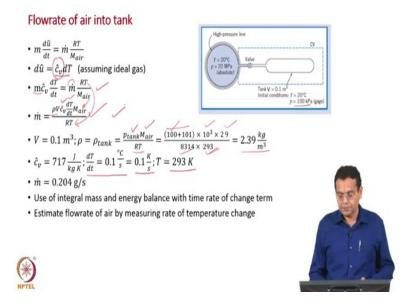
So, now we are almost few more steps to find out the flow rate of air into the tank that is equation which we have written in the last slide.
