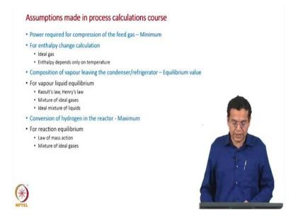
Now, for calculating the power required for compression of the feed gas, we said we will get the minimum power required. This power required is calculated from enthalpy change. So, in a process calculation course, we assume that the gas is ideal and hence we assume the enthalpy to depend on the temperature only. So, based on the assumption that it is an ideal gas and the enthalpy depends on temperature only we will find out what is the power required.
