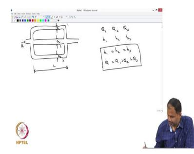
So, let us take an example. So, let us say you have a fluid that is entering the pipe and let us its divided into 3 parts ok. So, the pipe is divided into 3 parts ok. So, let us call the first 1 pipe 1, pipe 2 and pipe 3, all of them let us say have a length L and let the diameter be different.
