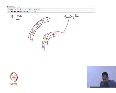
Let us say a bend in the pipe or an elbow that you will collect. For example, you need to take the pipe like this and then take a corner and go. Why would that cause additional losses? Something here the fluid is going like that. It could be a sharp 90 degree bend or
