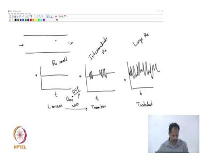
We have a let us say two plates and there is a fluid flow in it. And let us say you are interested in finding out what is the velocity and to find out velocity you actually you are going to do an experiment and you are going to put a probe a velocity probe to measure velocity at a particular point let us say.
