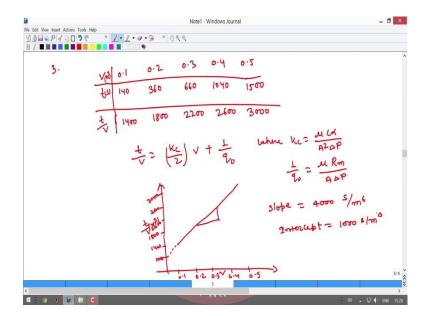
Now, I am going to solve the 3rd question in this tutorial. In the 3rd question I e filter has an area of 0.5 metre square and operate at a constant pressure drop 500 kilo Pascal. The following test result were obtained for slurry in water which gave raise into a filter gate the table is given here, volume versus time. 0.1, 0.2, 0.3, 0.4, 0.5, 140 second meter cube 360, 660, 1040, 1500 this is also a constant pressure programme. So, we are going to apply the same equation as in the first one.
