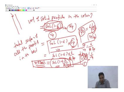
Let me just go back here what is the volume of solid particles in the column, what is that? It is going to be S 0 which is the cross section area times L that is going to give me the volume of the packed bed that multiplied by 1 minus epsilon is going to give me the volume of the solids in the is that. That is going to give me what is the total volume of all the solid particle that you have in the packed bed.
