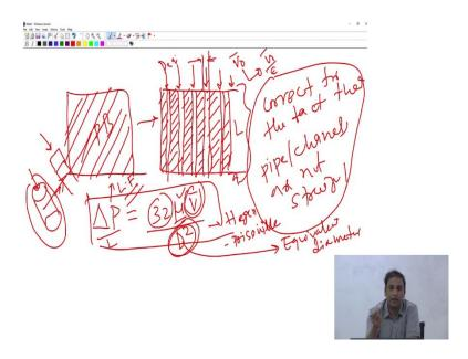
Now, the way we are going to work out this channel model is that, we are going to say that I am going to replace a complicated packed bed with a very simple configuration where I am going to say that there is a channel for the liquid to flow through and you have this the hatched region that I am that I am drawing these are the solids that formed the packed bed; of course, is a very simplified model right.
